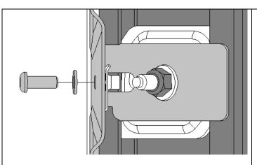
9. Secure each of the 4 mounting plates to the air deflector. Use the M6 Button head screws and black M6 washer (part# 4584329) as shown.
